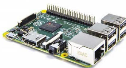
Figure 3. Raspberry Pi 2 Modelo B [FOUNDATION. 2015].
